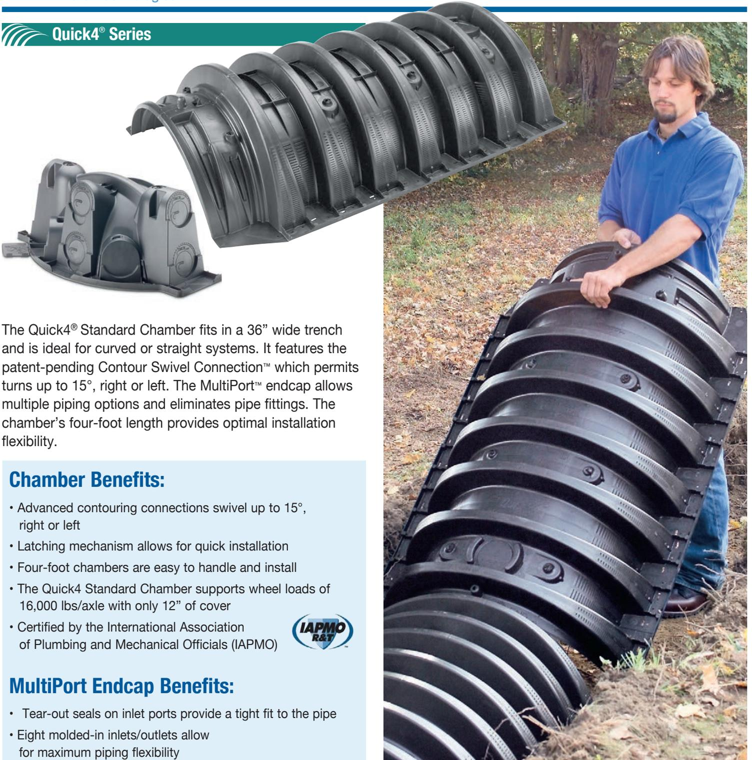
The Quick4® Standard Chamber fits in a 36" wide trench and is ideal for curved or straight systems. It features the patent-pending Contour Swivel Connection™ which permits turns up to 15°, right or left. The MultiPort™ endcap allows multiple piping options and eliminates pipe fittings. The chamber's four-foot length provides optimal installation flexibility.
